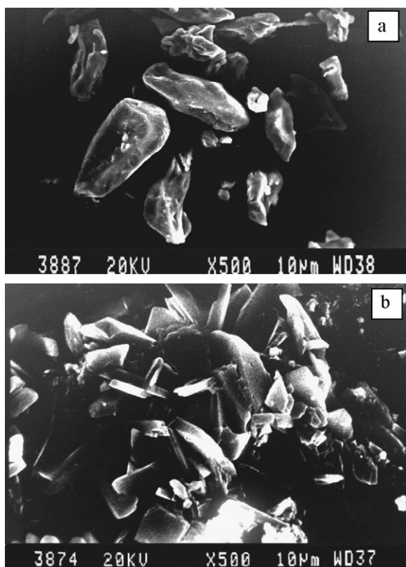
Fig. 2. SEM of (a) ungrafted guar gum and (b) grafted guar gum.
